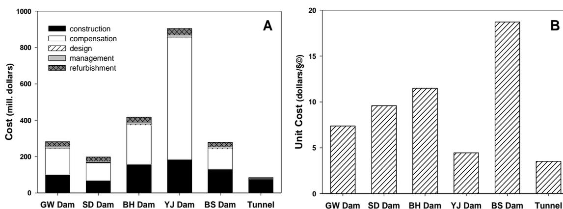
Fig. 2. Comparison of economic efficiency in relation to water supply quantities between the new dams and the Connecting Tunnel (A) Contents cost, (B) Unit cost per water supply
