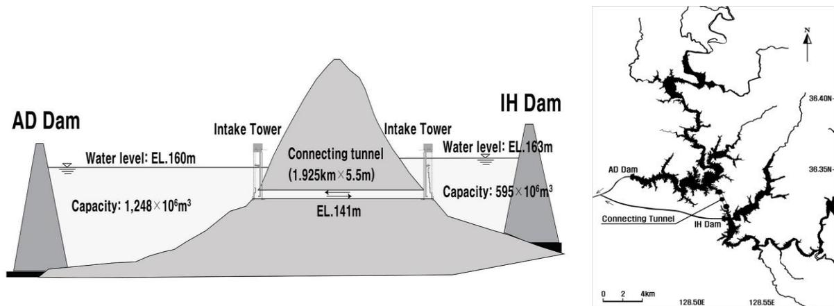
Fig. 1. Mimetic diagram of the Andong(AD) Dam-Imha(IH) Dam Connecting Tunnel (K-water, 2011)
