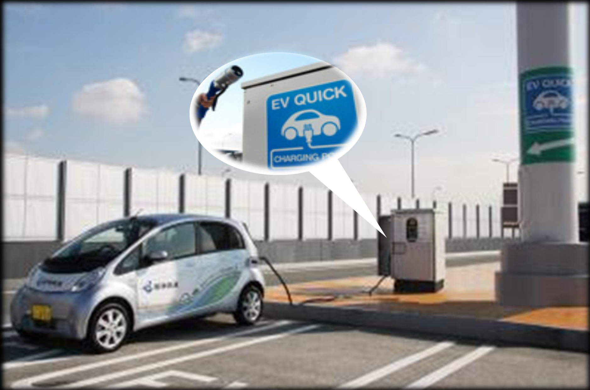
EV Model Car of HEC with the Rapid Battery Charger at the Nakajima Parking Area along the Hanshin Expressway
