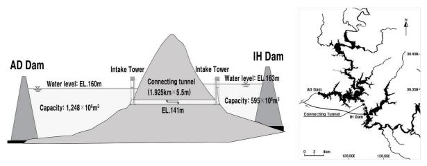
Fig. 1. Mimetic diagram of the Andong(AD) Dam-Imha(IH) Dam Connecting Tunnel (K-water, 2011)
