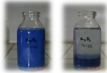
Figure 1. Turbidity of batik effluent before and after treatment with 40000 mg/l coagulant of M. oleifera seeds and deposition length of 180 minutes.
