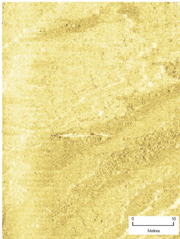
70657: Sidescan sonar image of Wreck 70657 18.5m x 6.2m x 0.9m
