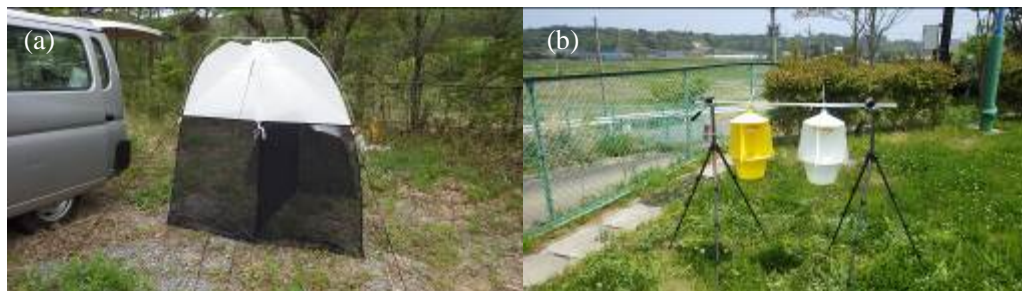
Fig. 3 (a) Malaise trap and (b) flight intercept trap for monitoring flying insects such as pollinators
