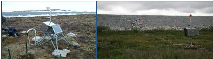
Thermal data capture stations on the permafrost at Tasiujaq airport
